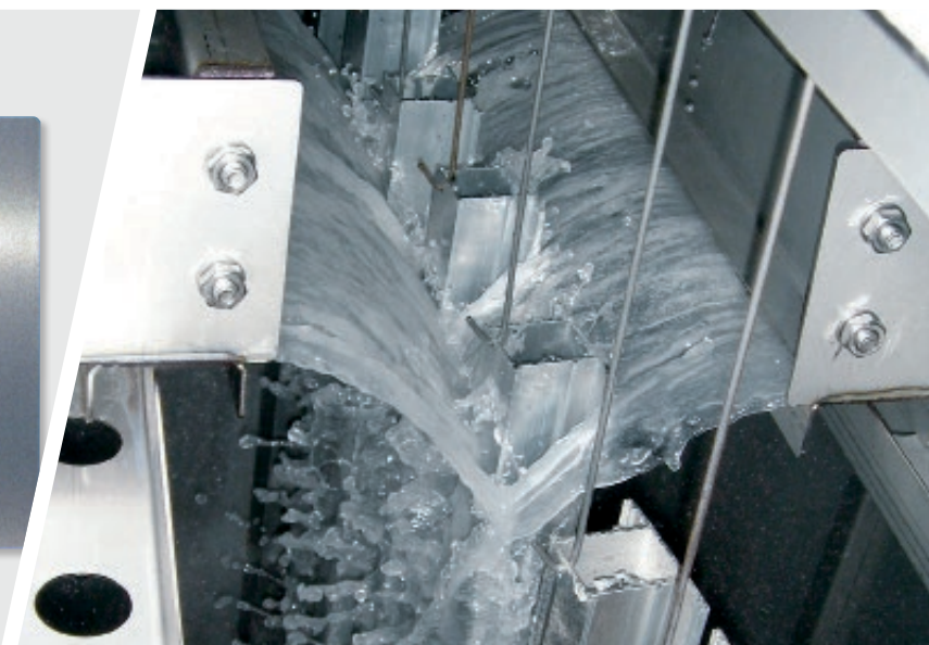
Gardobond® X 4707 for the passivation of aluminum sections in a vertical plant
