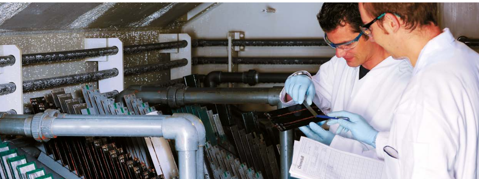
Walk-in salt spray chamber at the Chemetall laboratory.
